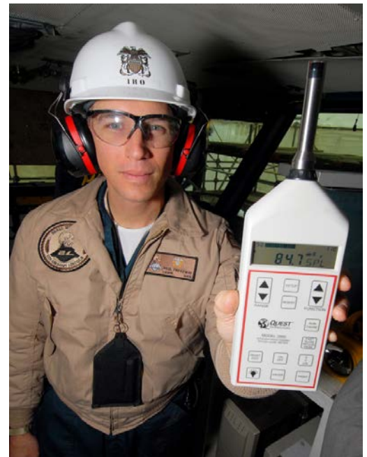
A Navy officer uses a sound level meter to test for high decibel levels. Image retrieved from Bing Images (free to use and share license)
